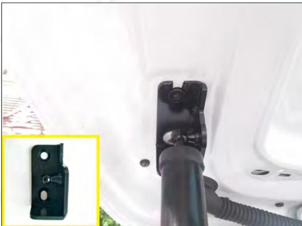
5. Remove the original left upper bracket and the brace rod. Install our upper left bracket (**The ball head position is facing outward**). and fix it with our screws.
