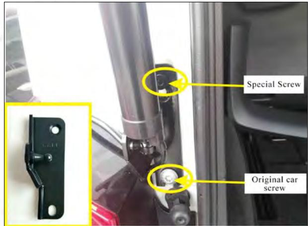
4. Remove the original left lower bracket and the brace rod. Install our lower left bracket (**The ball head position is facing inward**). The top of the bracket is fixed with our screws, and the bottom is fixed with the original car screws.
