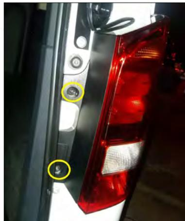
6. Remove the two screws in the yellow circle and remove the car lights (The left and right steps are the same).
