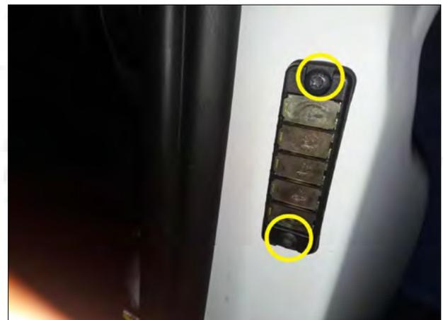
11. Remove the trim panel from the main driving belt B column and find this socket. Then remove the screw and this socket.
