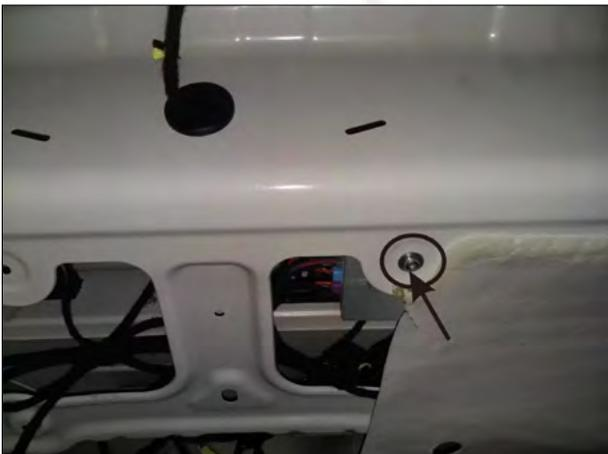
17. Remove the original car lock and add a gasket under the original car lock.
