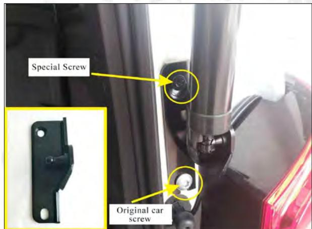
2. Remove the original right lower bracket and the brace rod. Install our lower right bracket (**The ball head position is facing inward**). The top of the bracket is fixed with our screws, and the bottom is fixed with the original car screws.
