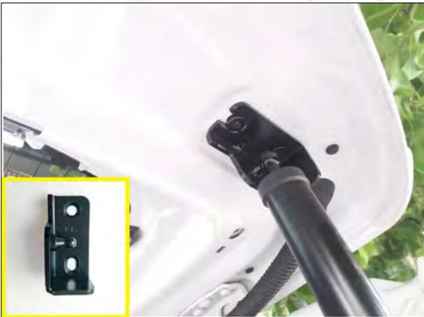
3. Remove the original right upper bracket and the brace rod. Install our upper right bracket (**The ball head position is facing outward**). and fix it with our screws.
