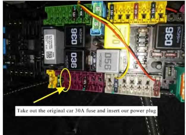
9. Remove the trim panel under the copilot to find the power supply, unplug the original car 30A fuse. Plug in our power plug.
