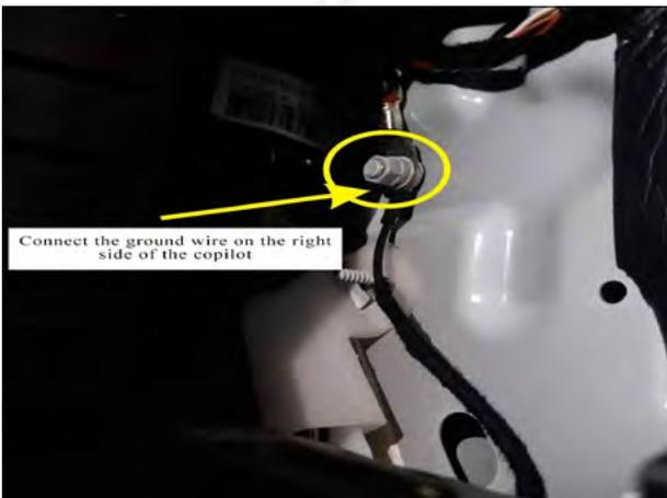
10. Find the ground wire on the right side of the copilot and connect the ground wire.
