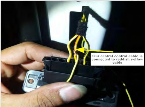
12. Our central control cable is connected to the reddish yellow cable of this seat (The third hole in the first row from left to right)
