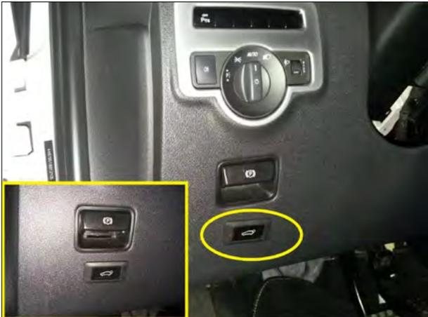
8. Remove the trim panel from the main driving, punch holes and install our front switch button.
