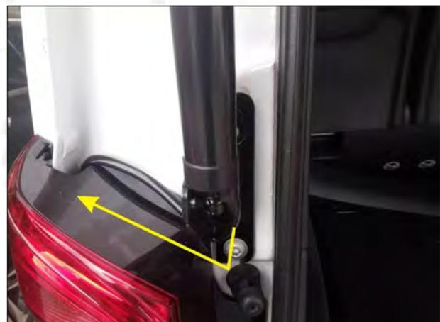
7. The brace rod cable is routed from the headlights to restore the lights (The same steps are left and right).
